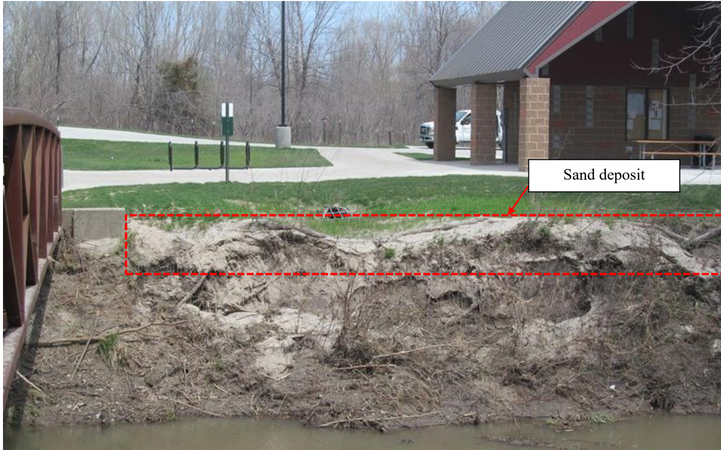
Figure 7.2 Clear Creek bank soils. Fresh sand was deposited on the flood plain at site 2 after a flood event.
