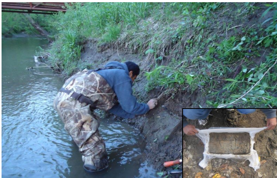
Figure 6.10 Sample extractions. (a) A sketch of the sample extraction scheme applied for the left and right banks at site 1 and 2. Figure not to scale. (b) Extraction of soil blocks from the right bank, cross section CC 1 at site 2. Inset: Soil was wrapped in cheese cloth before being transported from the field to the laboratory.
